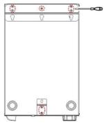
**Step2:** Mark the installation position with the mounting plate 1. The distance between the two mounting holes is 300mm.
